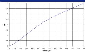
Note: Power Compression Losses were calculated after 5 minutes period applying a pink noise signal filtered between 25 and 200 F
